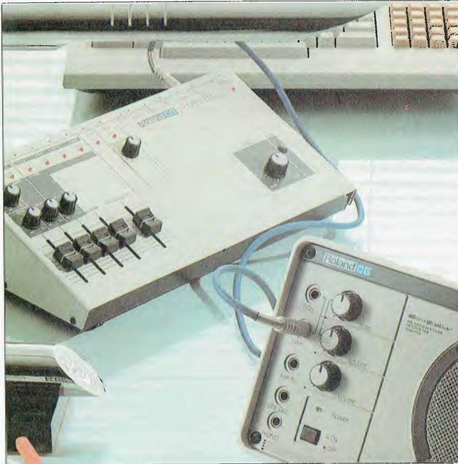
The CMU-800 Compumusic console from Roland, which hooks up to an Apple II or IIe.
