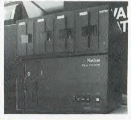
Right: Nashua's data conversion system, which copies data from 20 cm disks to 13 cm disks and vice versa.
